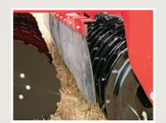
Trailed machines can be fitted with front discs in line with the subsoiling tines to reduce surface soil distur-
