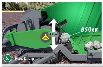
The lifting drum's power transmission is mounted along the drum frame, allowing the frame and the entire lifting drum to yield upwards, which makes it possible to lift stones 50 cm in diameter.
