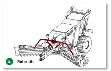
The lifting action is achieved with a hydraulic cylinder, which raises the rakes simultaneously. Mechanical locks secure them into the top position. The operator is able to position the picker in working or transport position from the cab.
