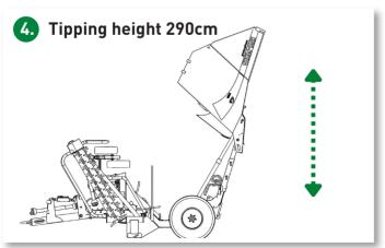
Tipping height is 290 cm(115") so emptying the stone container to larger trailers is easy. The lifting action is achieved with a hydraulic cylinder, which raises the rakes simultaneously. Mechanical locks secure them into the top position. The operator is able to position the picker in working or transport position from the cab.
