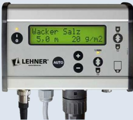
The menu of the AUTO-DOSIS control unit contains spreading charts from the manufacturer. If necessary, the manufacturer can install further spreading charts (if available).
